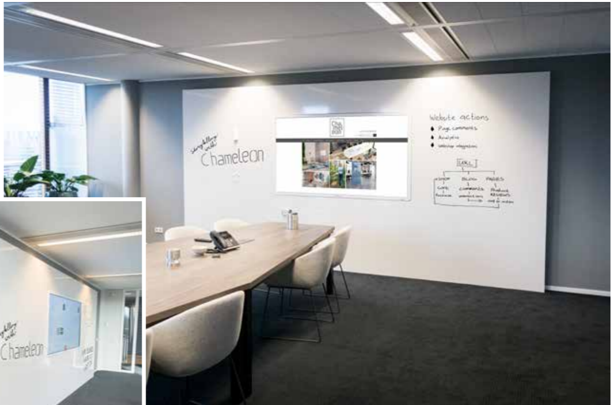
Writing wall with cut-out for display Writing surface: white enamel Finish: white laquered edges, right-angled corners. Cut-out with the same radius as display (R=8). Sides are finished with strips of whiteboard. Wall dimensions: 490 x 248 cm (W x H)
